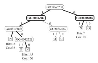
**Fig. 1.** Example of a Random Tree used to calculate the statistics  $Prec_{GO.0006887+N}$ . In this tree, leaf nodes (where a prediction is made) are represented by squares with the predicted class in it, edges in bold form the relevant rules (a rule is a path from the root to a leaf node). We also show the OOB Hits and Coverages that are relevant to calculate the statistics  $Prec_{GO.0006887+N}$
