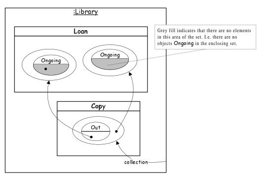
Figure 11: Constraint diagram for invariant 4
