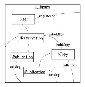
Figure 2: Instance diagram not satisfying constraint, but satisfying type diagram
